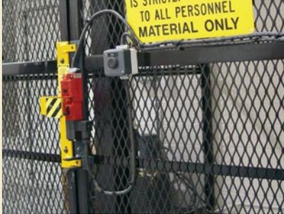
All Beech MATERIALIFT® VRCs meet the ANSI/ASME B20.1-2000 safety standard for conveyors. We can supply all required safety enclosures and gates with interlocks, as well as further safeguards (such as automatic load stops to contain off-balance or rolling loads). Just ask your Beech representative for further details. And remember: MATERIALIFT® VRCs are for material loads only!
